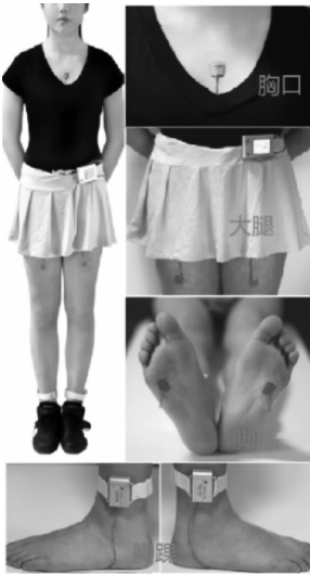
图1 受试者便携式步态分析仪佩戴方法示意图 Fig.1 Schematic diagram of the subject wearing IDEEA
